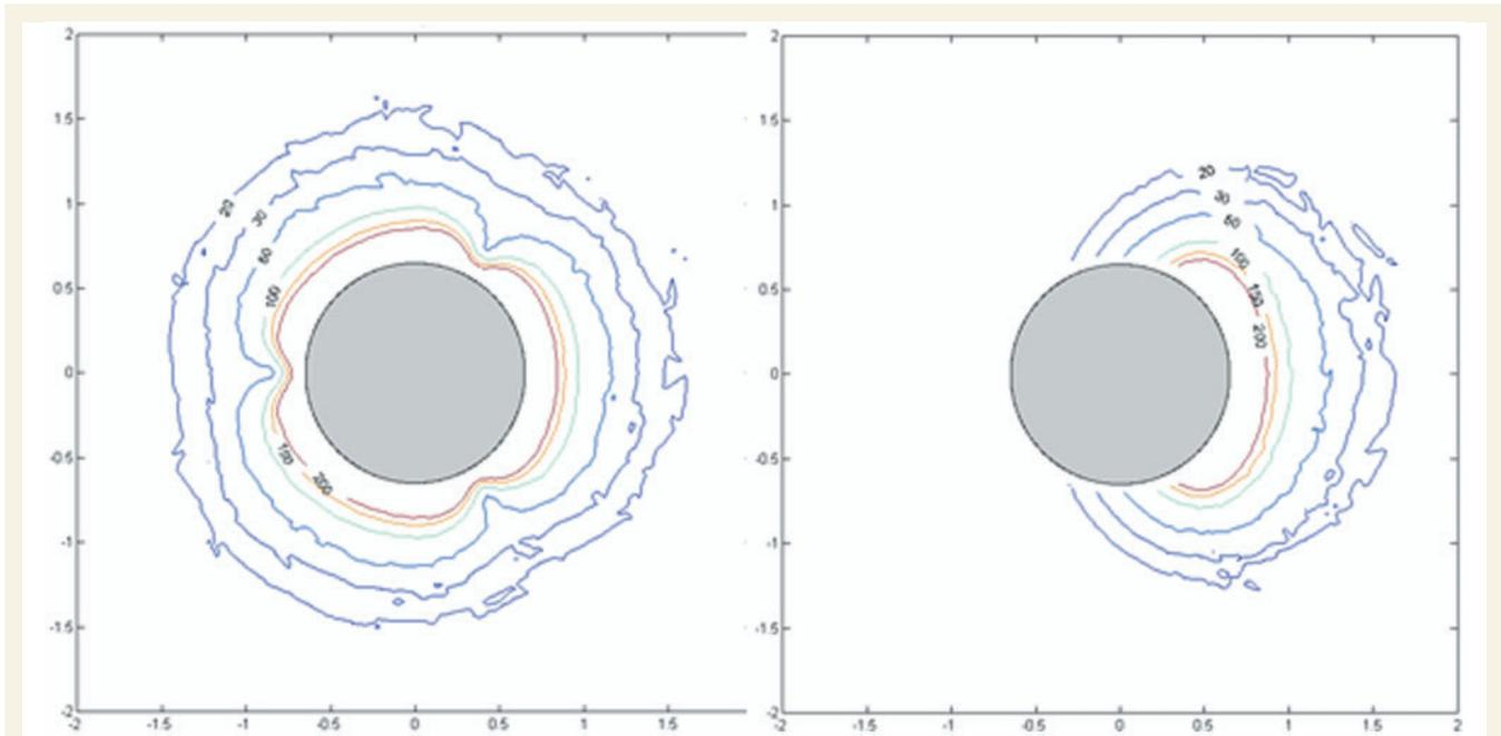
**Figure 4** Transverse view of activated tissue volume isolines, when 1-V stimulation is applied. *Left:* All three electrodes simultaneously activated. *Right:* One-directional electrode activated. The disc represents a cross-section of the lead. The x- and y-axis labels represent millimetres from the centre of the lead.
