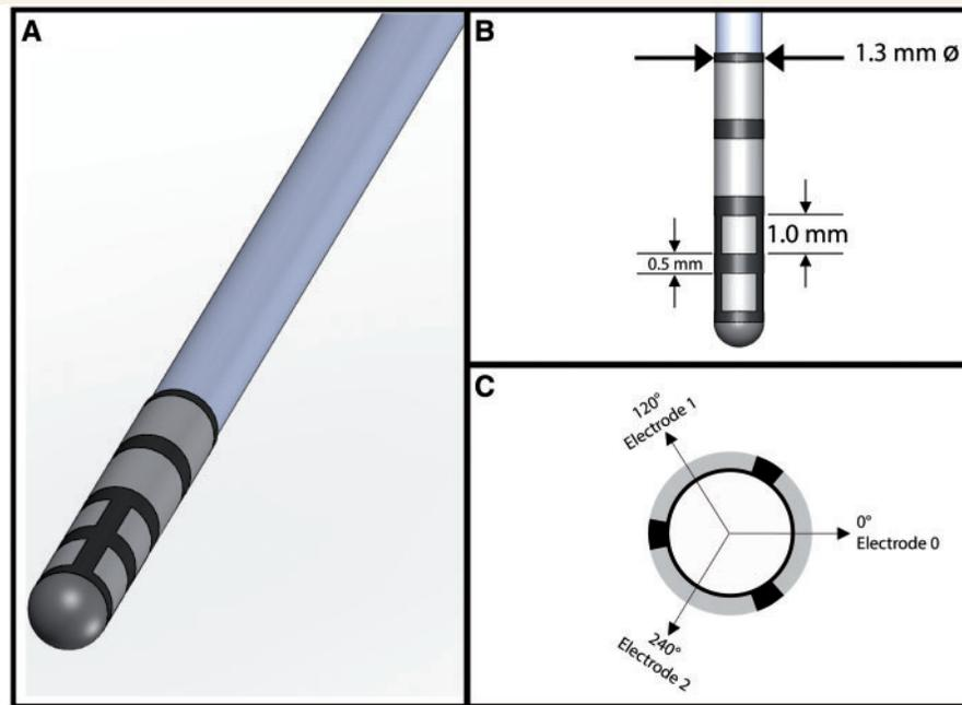
**Figure 1** Distal end of the directSTNacute lead. (A) 3D representation. (B) Longitudinal view showing the dimensions of the directional electrodes and spacing. (C) Axial view with angles of direction.
