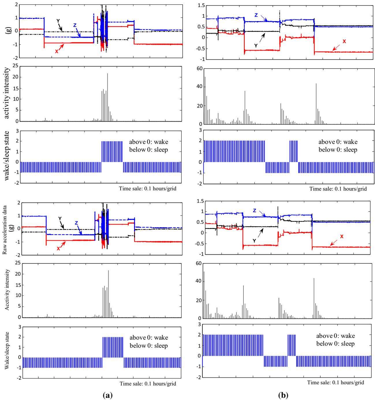
**Fig. 3** Raw acceleration data, activity intensity, and identified states during 1 h for **a** wrist algorithm and **b** chest algorithm
