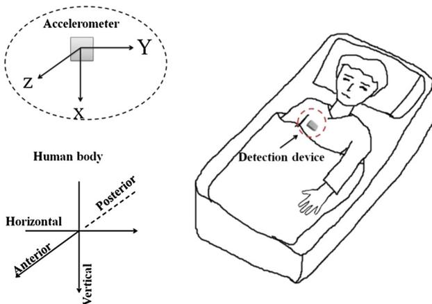
Fig. 6 Orientation of accelerometer relative to human body
