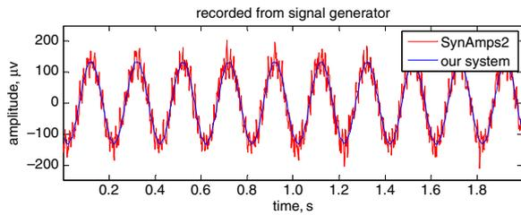
**Fig. 3** Raw waveforms recorded from signal generator
