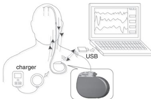
Fig. 1 Application example and system partition for prototype
