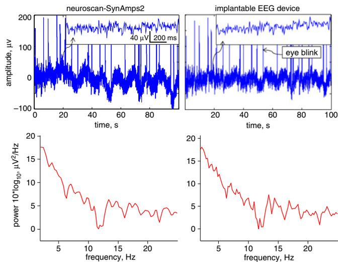
**Fig. 4** Synchronously acquired time-domain raw waveforms and spectrums of two systems
